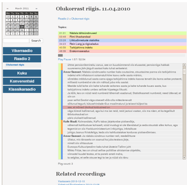
Figure 2: Example screen of the TSAB system. Shown is the view of a single recording, with the recording directory on the left, topic segmentation of the recording at the top, transcript segmented by speakers and topics in the middle, and links to automatically found semantically similar recordings near the bottom. See http://bark.phon.ioc.ee/tsab .
